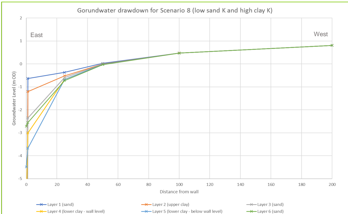
Plate 3.3: Worst Case Groundwater Drawdown (Scenario 8) with Distance from Cofferdam for each Model Layer
